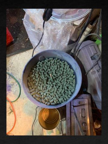
By using a brass tumbler, more cast bullets can be easily powder coated to speed up the process.
