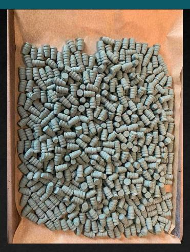
Once bullets are coated, they are dumped into a wire fry basket so excess powder can be shaken off. Then, they are placed on a baking tray with parchment paper.
